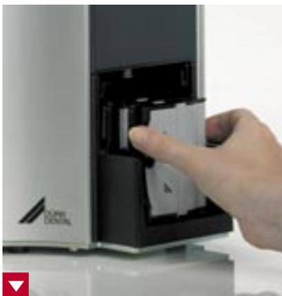
▼ The fully automatic transport system presents the scanned and deleted image plates in the cassette.
